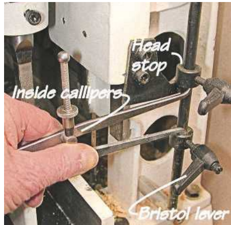
▲ Pic.6 The stops are difficult to reach, so Jeff had to use callipers to set the mortise depth
